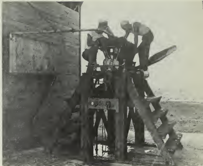
MOTORMEN —Forerunners of today's Aviation Machinist's Mates check engine in test stand at Pensacola in 1917.
